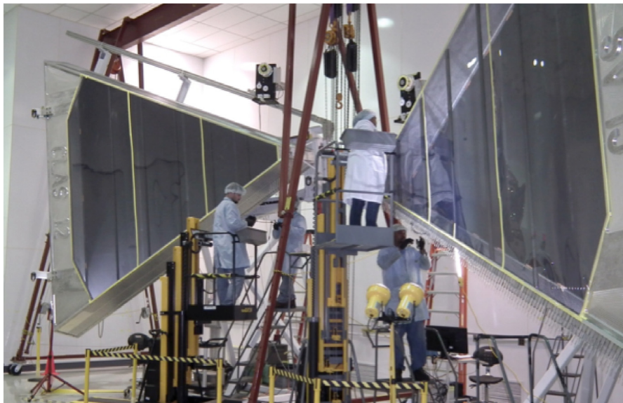
Fig. 13. Simultaneous wire stringing of two R3 chambers in the Jefferson Lab clean room.
